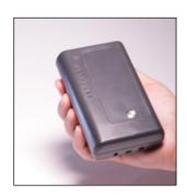
The microAeth® MA200 is a compact, real-time, wearable 5-wavelength UV-IR Black Carbon monitor with a 15 sampling location automatic filter tape advance system which allows for up to 2-3 weeks of continuous measurements.
