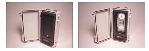
The microAeth® MA350 is a real-time 5-wavelength UV-IR Black Carbon monitor housed in an outdoor-rated case with an 85 sampling location automatic filter tape advance system which allows for 3-12 months of continuous measurements.
